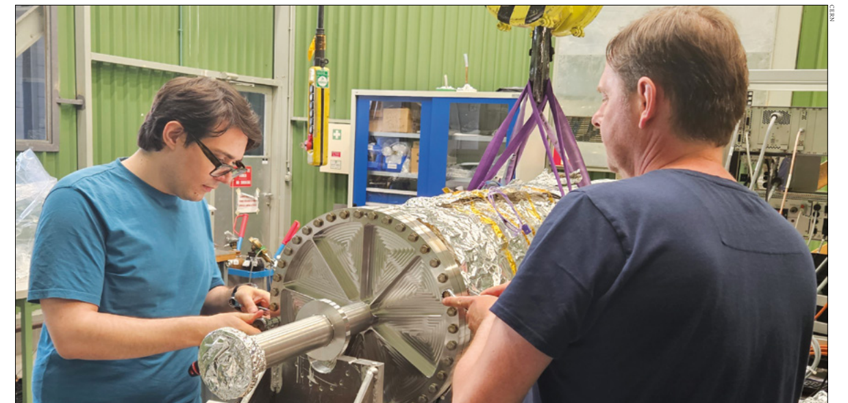
Project planning Two CERN groups are engaged as contributing partners on the beampipe studies for the Einstein Telescope – specifically, the vacuum, surfaces and coatings (TE-VSC) and mechanical and materials engineering (EN-MME) groups. Above: CERN members of the Einstein Telescope beampipe study teams install the first pre-prototype beampipe demonstrator.
