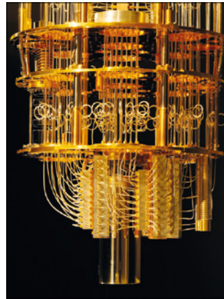
Quantum potential A quantum computer built by IBM based on superconducting qubits.
