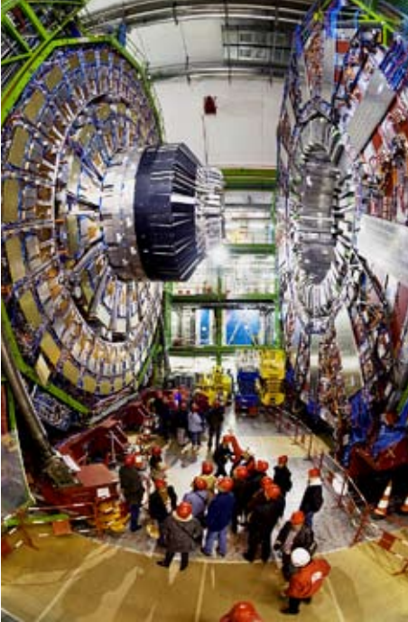
Figure 4. Central part of the CMS detector. The left half shows part of an endcap muon system. Muon chambers are visible as the copper colored trapezoidal boxes. Ohio State-built electronics are mounted on the chambers inside electrostatic shields.
